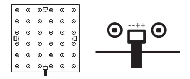
Please note that the starter cable must be connected to an orientation that shows "- - + +".
